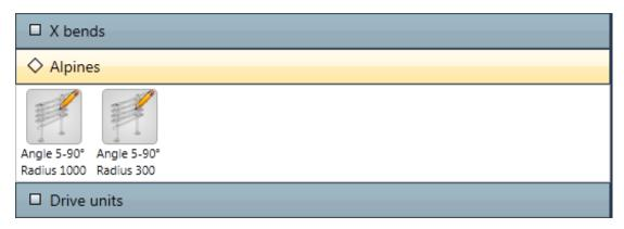
The alpine have 3 editable properties; slope angle, number of levels (n) and the cc distance (distance between center points of the wheel bends).
