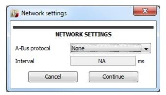
The Network settings window should in the stand-alone case be set to *None*. If an external network is to be used this is specified here. *CANopen*, *DeviceNet*, *Ethernet/IP or Profinet* are possible options.
