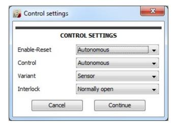
The last popup window in the wizard is the control settings window. The first two choices (Enable-Reset and Control) could not be set to anything else than *Autonomous* if no network was selected
