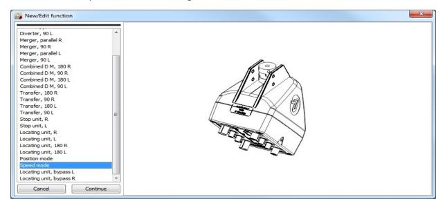
The next window in the wizard decides which standard (physical) type the unit should be set to if it is a part of the X45e platform. But there is also two generic control options, Position mode and Speed mode. The **Speed mode** option should be selected in this case.
