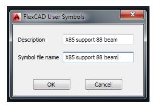
The objects that were chosen to be part of the user symbol are removed from the drawing and the function window is closed. To insert the symbol into the drawing, start the function again. The *FlexCAD User Symbols* window opens and in the top left part of the window, look up the symbol and then click *Insert*, see picture below. The *FlexCAD User Symbols* window closes and the symbol is at the cursor and it can be placed where ever the user wishes.
