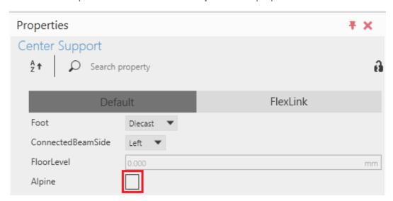
When the check box is ticked options will be presented where the number of brackets and the height of each bracket can be set. The height of each bracket is calculated from the first bracket in the bottom of the support. This bracket should always be connected to the lowest level in the alpine. Before adjusting the brackets connect the support and select the number of brackets needed by changing the value of the property **NbrOfBrackets**.
