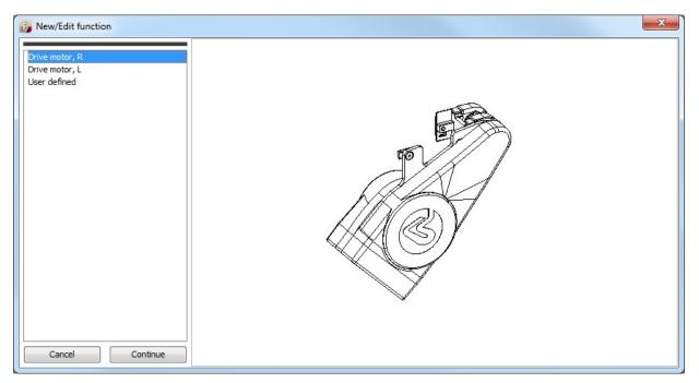
The next window in the wizard decides which (physical) type the unit should be set to. For a conveyor unit it has only two alternatives, the left or the right version, and the **User Defined** version. The later option is not automatically setting the other parameters but leaves this to the user. The right and the left version only differs by the sign of the speed setpoint. This setpoint can be changed later from the settings window.
